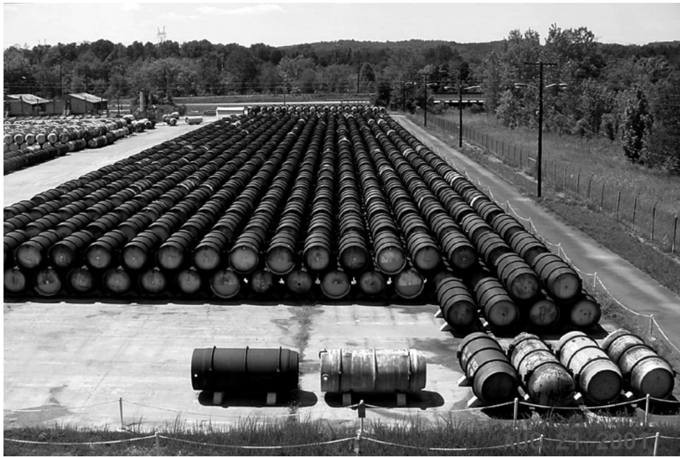
Figure 4.3. Cylinders of depleted uranium at the storage area at the K-25 site, Oak Ridge, Tennessee, in 2001. The site held over 6000 cylinders containing depleted uranium “tails” produced as waste by the gaseous diffusion enrichment plant, which was closed in 1964 and is now being demolished. Beginning in 2002, these particular cylinders were
