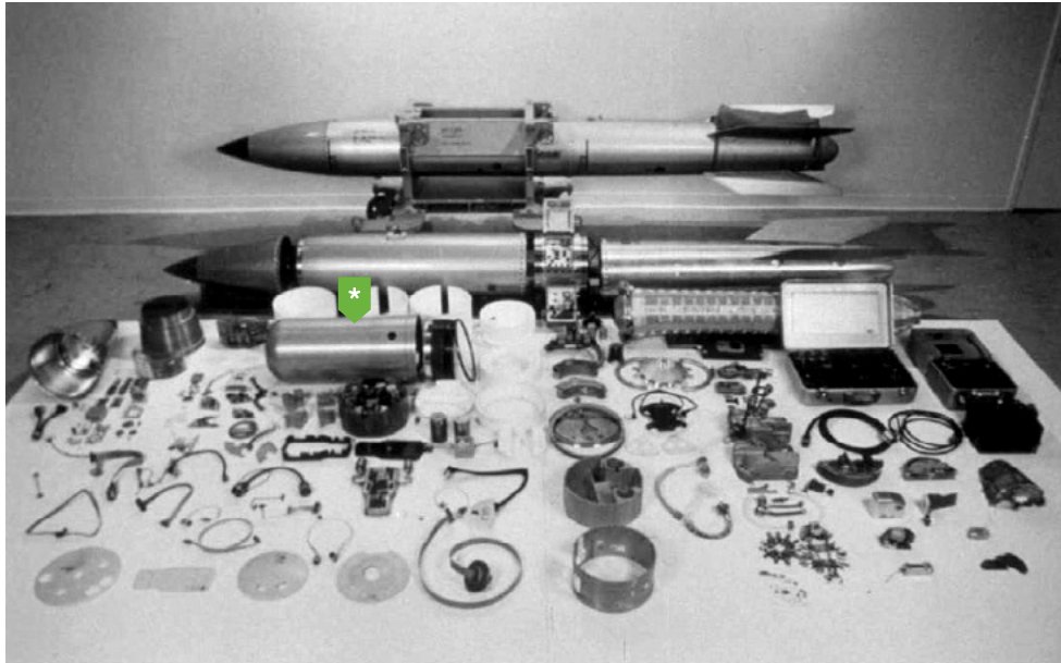
Figure 3.6. Components of a U.S. B-61 thermonuclear weapon. A nuclear weapon is a complex mechanism, with the nuclear explosive or “physics package” (*) and its associated arming, fusing, firing and safety systems. The physics package is itself a composite, made up of a plutonium shell or
