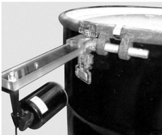
Figure 5.7. Seal with integrated identity tag and small battery-operated electronic camera that transmits the image continuously. 243
